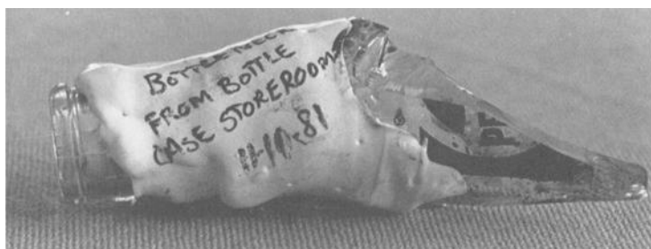
FIG. 14—Silicone ( Dent-Kote insulating paste) poured over broken bottleneck. Bottleneck was processed with fingerprint powder before pouring the silicone.
