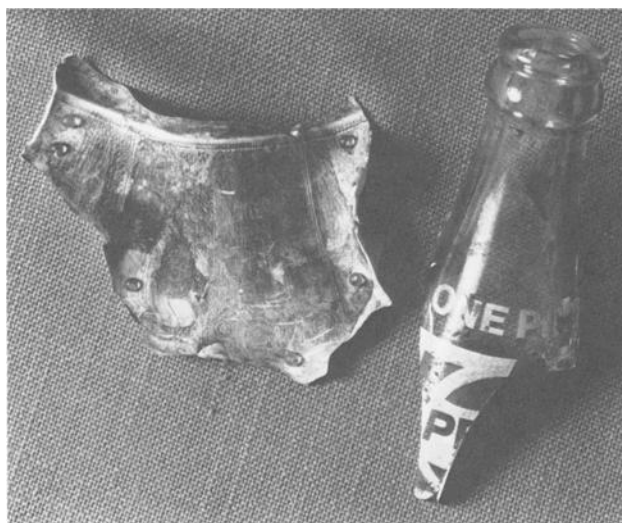
FIG. 15—Silicone cast and bottleneck. Note that cast is reverse or negative image.
